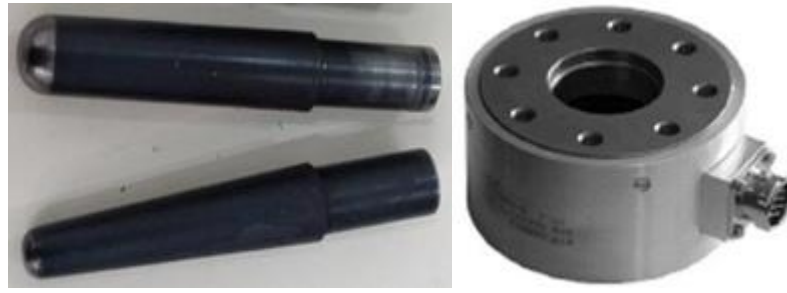
Figure 3. The tool steel punches ( d = 10 and 15\text{mm} ) and the multi-component force transducer FN73252
