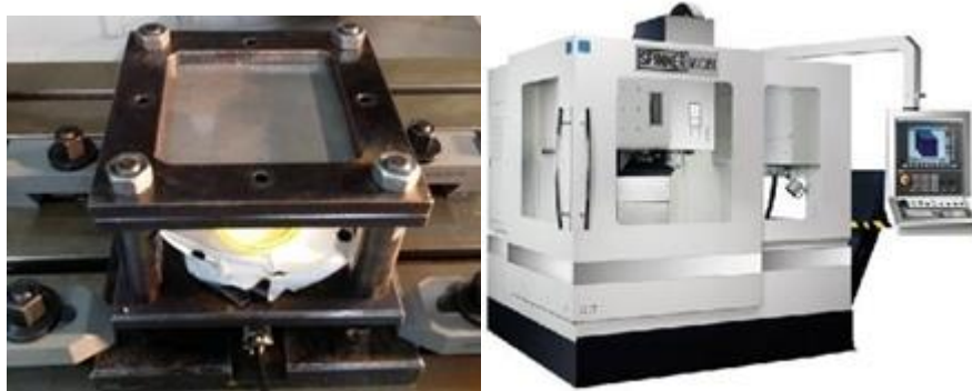
Figure 2. CNC Spinner MCV8501 machining center and SPIF incremental forming device
